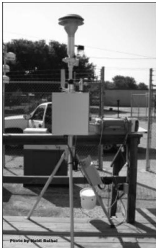
Figure 8. E-BAM installed at Clinton Drive. Picture from Mayor’s Task Force Report on the Health Effects of Air Pollution.
